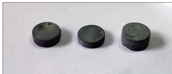
Fig.2. compacted pure silicon after pressing
