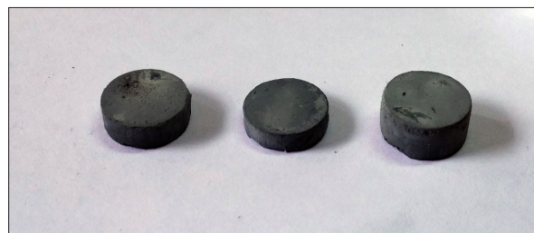
Fig.2. compacted pure silicon after pressing
