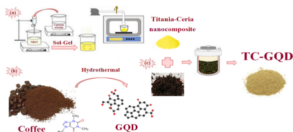
Fig. 8. Schematic presentation of preparation processes for TC-GQD
