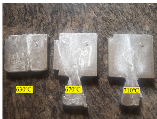
Fig. 2. Cast samples of composite prepared at different temperatures.
