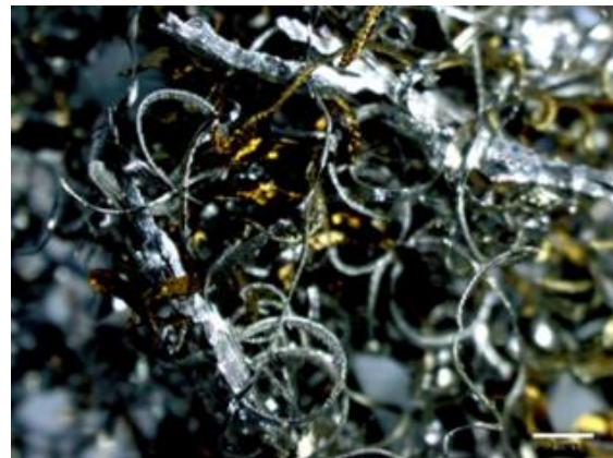
Fig. 1. AA 7075 swarf produced from the machining process
