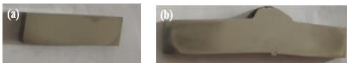
Fig. 2. Images of samples used in present study: base metal (BM) and welded sample
