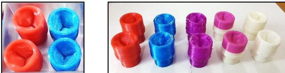
Fig. 10. The 3D printing of artificial tri-leaflet heart aortic valve (TAV) mechanical heart valve
