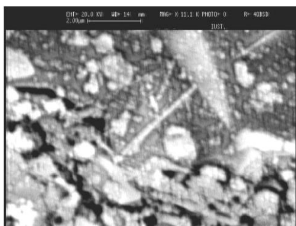
Fig. 6. Microstructure of sample without silica sol after sintering at 1400 °C showing no mullite crystals (figures 4-6), it can be concluded that the mullite
