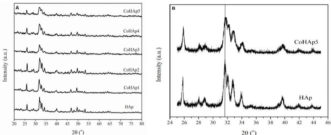
**Fig. 1.** (A) X-ray diffraction pattern of synthesized HAp, CoHAp1, CoHAp2, CoHAp3, CoHAp4 and CoHAp5
