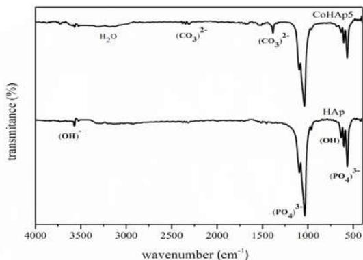
Fig. 2. FTIR spectrum of HAp and CoHAp5
