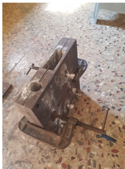
Fig. 1. Stir casting setup and Die used for preparing MMC
