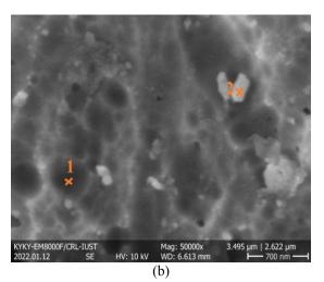
Fig. 3. a-b FESEM microstructure of the bulk hot-pressed Al5083 alloy at different magnifications.
