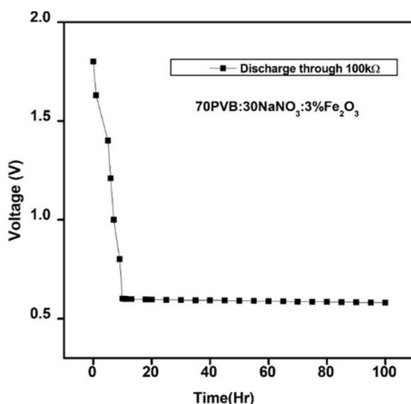
**Fig. 8.** Discharge properties of an electrochemical cell with a 70PVB+30NaNO<sub>3</sub>+3% Fe<sub>2</sub>O<sub>3</sub> polymer electrolyte (load= 100 kΩ)
