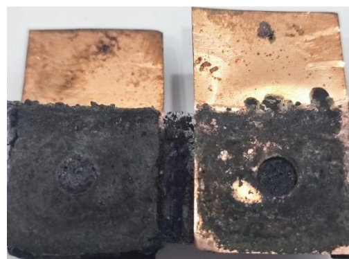
Fig. 12. Barrier layer formed between the sample surface and the electrode
