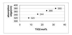
Fig. 3. adsorption edge wavelength with TiO<sub>2</sub> content.
