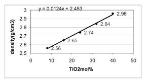
Fig. 1. glass density according to TiO<sub>2</sub> content.
