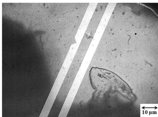
Fig. 7. Example hardness indentation on the cross section of a ribbon.
